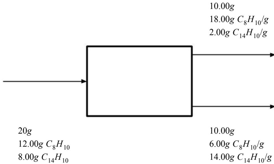
In scaling the end flow rate by 500 lb<sub>m</sub>/min, the initial entering flow must then be scaled by 1000 lb<sub>m</sub>/min to account for the two exit flows. This would be the resulting diagram:
