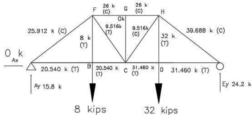
This first scenario was chosen as one of the “worst case scenarios” because it applies large loads on the members. The right side of this bridge, which only has one support reaction, has members that experience forces up to about 39 kips. Because of the high forces, some recommendations include using a strong material or increasing the number of members to make this bridge more reliable.
